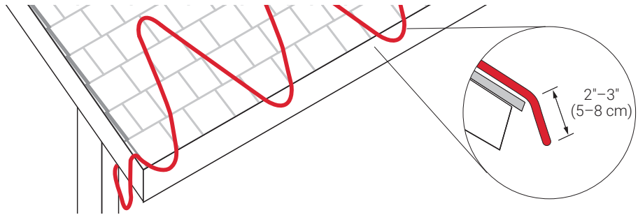
Figure 6 Layout for heated drip loops
