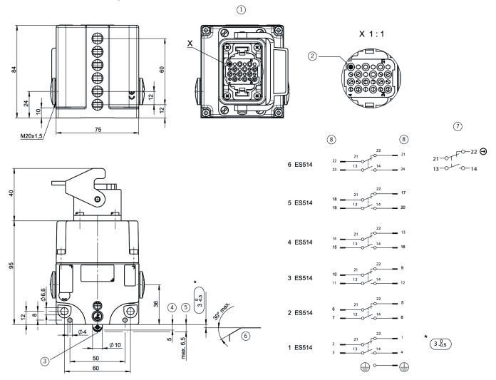
To obtain the direct opening travel, the trip dog setting distance must be maintained. Actuating \*elements such as cam approach guides must be firmly mounted, i.e. riveted, welded or otherwise secured against becoming loose.
