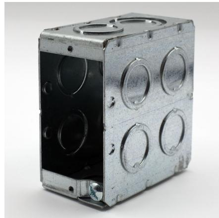
Masonry Box, 3-1/2 in. Deep, 21 Cu. In., 1-Gang Masonry Box, 2 in. Width, 3-3/4 Height, Raised ground screw, with Concentric, 1/2 & 3/4 in. KO (20-Pack)
