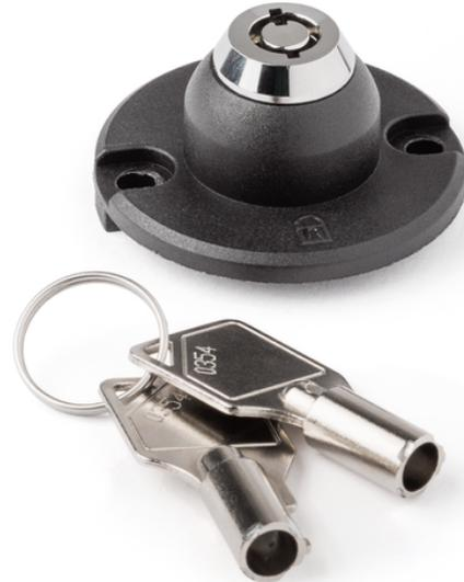
The lock is used in combination with safety switch CTP/TP/STP. The auxiliary key release enables authorized personnel to actuate the auxiliary release using the related key. The unlocking mechanism holds the solenoid in the “unlocked” position. 2 screws are used to fix the lock to the cover of the safety switch (above the auxiliary release).
