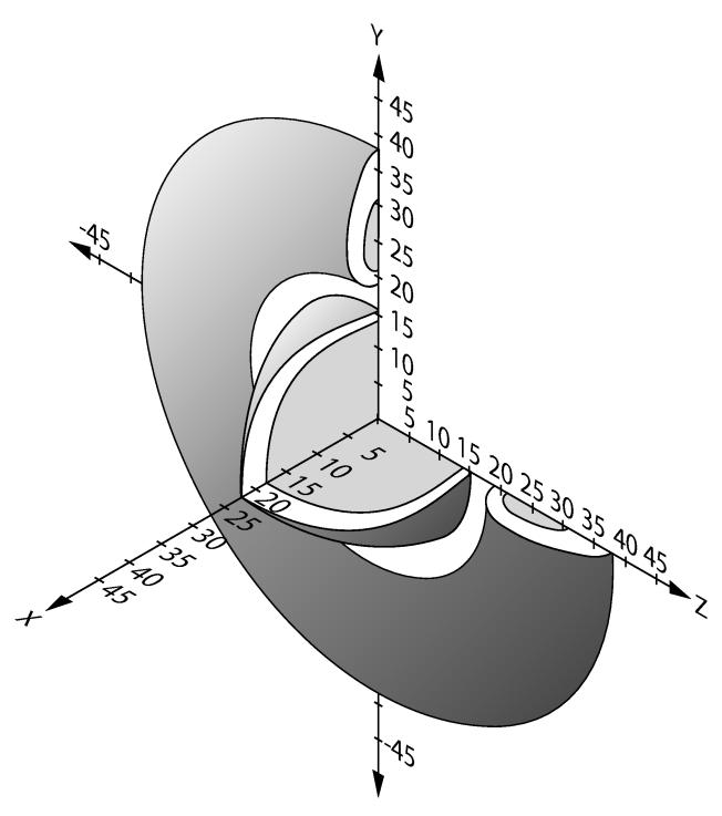
For a side approach direction for the actuator and safety switch, a minimum distance of s = 6 mm must be maintained so that the actuating range of the side lobes is not entered.
