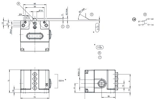
Safety switching element ES514 positive opening. Positive opening function is dependent on maintaining this distance.
