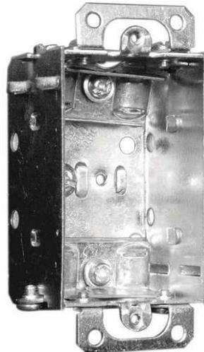
Single Gang Device Box, Gangable, 1-1/2 in. Deep, 8 Cu. In., with Raised Ground Screw, Flush Ears, Cable Pryouts Ends, NMD90 and AC90 (50-Pack)
