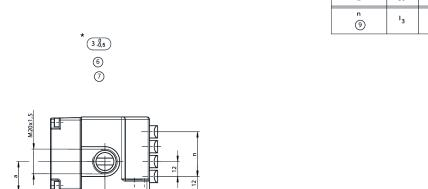
Safety switching element ES514 positive opening. Positive opening function is dependent on maintaining this distance.
