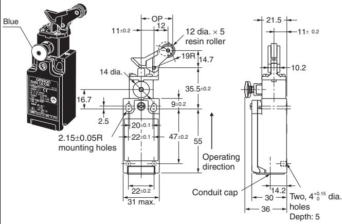
**Note:** Variation occurs in the simultaneity of contact opening/closing operations of 2NC, 2NC/1NO, and 3NC contacts. Check contact operation.
