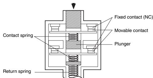
Conforms to EN60947-5-1 Direct Opening (Both NC Contacts have a direct opening mechanism.)
