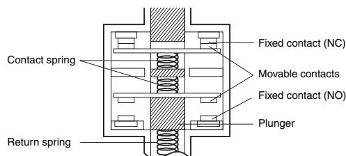
Conforms to EN60947-5-1 Direct Opening (Only NC Contact has a direct opening mechanism.)
