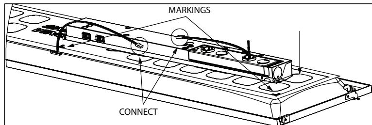
**Step 5:** Engage the hinge hooks on each end of the CPXR Kit into the corresponding slots in the Adapter Brackets and slide completely down both slots.
