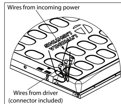
**Step 7:** Close and latch CPXR Assembly door, making sure no wires are pinched or exposed. Turn ON power at circuit breaker and test successful installation.
