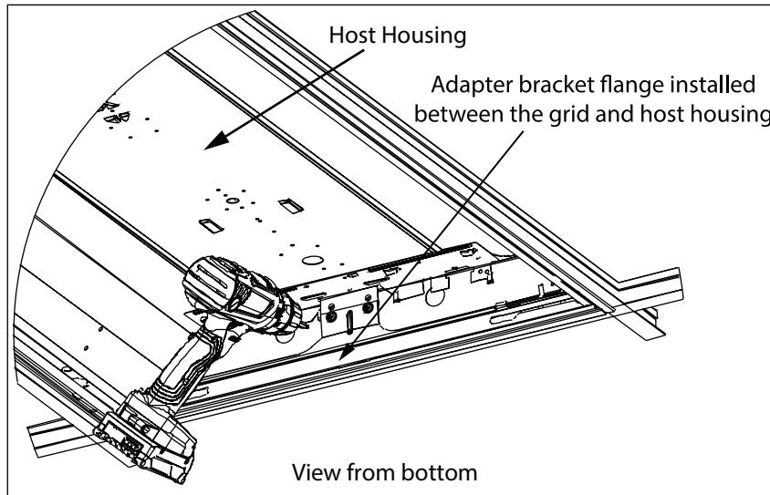
**Step 3:** Install the included trim strips on each side of the opening by sliding the flat flange of the strip between the T-Grid and the host housing to secure.
