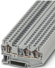
Feed-through terminal block, nom. voltage: 800 V, nominal current: 32 A, number of connections: 3, connection method: Spring-cage connection, Rated cross section: 4 mm<sup>2</sup>, cross section: 0.08 mm<sup>2</sup> - 6 mm<sup>2</sup>, mounting type: NS 35/7,5, NS 35/15, color: gray
