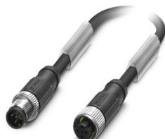
Sensor/actuator cable, 5-position, PUR halogen-free, black-gray RAL 7021, shielded (Advanced Shielding Technology), Plug straight M12, coding: A, on Socket straight M12, coding: A, cable length: 0.6 m
