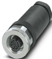
Connector, Universal, 8-position, Socket straight M12, coding: A, Screw connection, knurl material: Brass, nickel-plated, cable gland Pg9, external cable diameter 6 mm ... 8 mm
