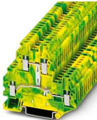
Protective conductor double-level terminal block, number of connections: 4, connection method: Screw connection, cross section: 0.14 mm<sup>2</sup> - 4 mm<sup>2</sup>, mounting type: NS 35/7,5, NS 35/15, color: green-yellow
