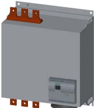
SIRIUS soft starter Values at 575 V, 50 °C standard: 615 A, 700 hp Inside-delta: 1065 A, 1200 hp 400-600 V AC, 115 V AC Screw terminals !!! Phased-out product !!! Successor is SIRIUS 3RW5, Preferred successor type is >>3RW5553-6HA16<<
