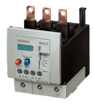
Overload relay 22...32 A For motor protection Size S3, Class 10 Contactor mounting Main circuit: Screw terminal Auxiliary circuit: Screw terminal Manual-Automatic-Reset !!! Phased-out product !!! Successor is SIRIUS 3RU2 Preferred successor type is >>3RU2136-4EB0<<
