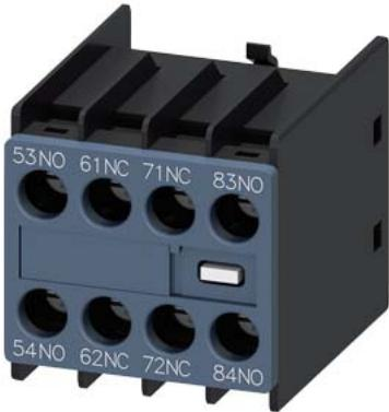
auxiliary switch, on the front, 2 NO + 2 NC, 53/54, 61/62, 71/72, 83/84, current path: 1 NO, 1 NC, 1 NC, 1 NO, screw terminal, physically coded, only with contactor relays 3RH2140 and 3RH2440 combinable (according to EN 50011)
