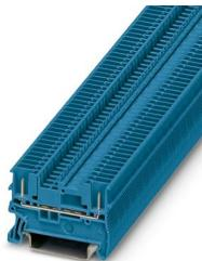
Feed-through terminal block, nom. voltage: 500 V, nominal current: 17.5 A, number of connections: 2, connection method: Plug-in connection, 1 level, Rated cross section: 1.5 mm<sup>2</sup>, cross section: 0.14 mm<sup>2</sup> - 1.5 mm<sup>2</sup>, mounting type: NS 35/7,5, NS 35/15, color: blue
