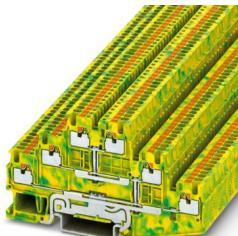
Ground terminal, nom. voltage: 500 V, nominal current: 15 A, connection method: Push-in connection, 1 level, Rated cross section: 1.5 mm<sup>2</sup>, cross section: 0.14 mm<sup>2</sup> - 1.5 mm<sup>2</sup>, mounting type: NS 35/7,5, NS 35/15, color: green-yellow
