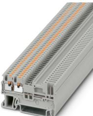
Feed-through terminal block, nom. voltage: 500 V, nominal current: 17.5 A, number of connections: 3, number of positions: 1, connection method: Push-in / plug connection, 1 level, Rated cross section: 1.5 mm<sup>2</sup>, cross section: 0.14 mm<sup>2</sup> - 1.5 mm<sup>2</sup>, mounting type: NS 35/7,5, NS 35/15, color: gray
