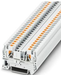
Feed-through terminal block, nom. voltage: 800 V, nominal current: 32 A, number of connections: 2, connection method: Push-in connection, Rated cross section: 4 mm<sup>2</sup>, cross section: 0.2 mm<sup>2</sup> - 6 mm<sup>2</sup>, mounting type: NS 35/7,5, NS 35/15, color: white
