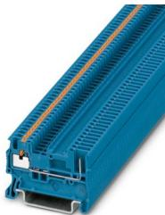
Feed-through terminal block, nom. voltage: 500 V, nominal current: 17.5 A, number of connections: 2, connection method: Push-in / plug connection, 1 level, Rated cross section: 1.5 mm<sup>2</sup>, cross section: 0.14 mm<sup>2</sup> - 1.5 mm<sup>2</sup>, mounting type: NS 35/7,5, NS 35/15, color: blue
