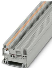
Feed-through terminal block, nom. voltage: 500 V, nominal current: 17.5 A, number of connections: 2, connection method: Push-in / plug connection, 1 level, Rated cross section: 1.5 mm<sup>2</sup>, cross section: 0.14 mm<sup>2</sup> - 1.5 mm<sup>2</sup>, mounting type: NS 35/7,5, NS 35/15, color: gray
