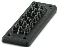
Cable feed-through plates, no. of conductors: 25, external cable diameter: 3x 3 mm ... 6 mm, 9x 3 mm ... 7 mm, 8x 6 mm ... 9 mm, 4x 6 mm ... 12 mm, 1x 10 mm ... 20 mm, material: PP (Core), material: TPE-SEBS (external material), color: black, length: 154 mm, width: 56 mm, height: 20 mm
