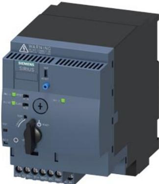
SIRIUS Compact load feeder Reversing starter 690 V 24 V AC/DC 50...60 Hz 3...12 A IP20 Connection main circuit: plug-in, without terminals Connection control circuit: screw terminal
