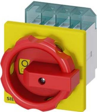
SENTRON, Switch disconnector 3LD, emergency switching-off switch, 3- pole, Iu: 16 A, operating power / at AC-23 A 400 V: 7.5 kW, front-mounted, rotary operating mechanism, Red / yellow, 4-hole mounting of the handle
