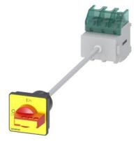
SENTRON, switch disconnector 3LD, EMERGENCY OFF switch, 3-pole, Iu: 63 A, Operating power / at AC-23 A at 400 V: 22 kW, floor mounting with door coupling, defeatable knob-operated mechanism, red/yellow, 4-hole mounting of the handle
