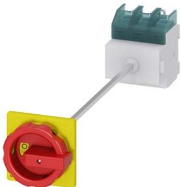
SENTRON, Switch disconnector 3LD, emergency switching-off switch, 3- pole, Iu: 100 A, operating power / at AC-23 A 400 V: 37 kW, floor mounting with door coupling, rotary operating mechanism, Red / yellow, 4-hole mounting of the handle
