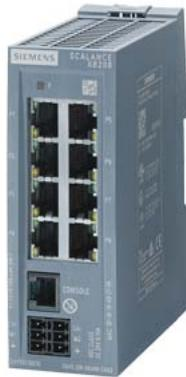
SCALANCE XB208 managed Layer 2 IE switch 8x 10/100 Mbit/s RJ45 ports 1x console port; diagnostics LED redundant power supply IEC 62443-4-2 certified; temperature range 0 °C to +60 °C; DIN-rail mounting; default PROFINET.
