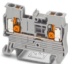
Feed-through terminal block, nom. voltage: 800 V, nominal current: 24 A, number of connections: 2, number of positions: 1, connection method: Push-X-connection, Rated cross section: 2.5 mm<sup>2</sup>, cross section: 0.5 mm<sup>2</sup> - 4 mm<sup>2</sup>, mounting type: NS 35/7,5, NS 35/15, color: gray
