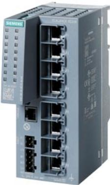
SCALANCE XC208 manageable Layer 2 IE switch; IEC 62443-4-2 certified; 8x 10/100 Mbit/s RJ45 ports; 1x console port; diagnostics LED; redundant power supply; temperature range -40 °C to +70 °C; assembly: DIN rail/S7 mounting rail/wall Office redundancy functions features (RSTP, VLAN,...); PROFINET IO device Ethernet/IP-compliant C-plug slot;
