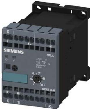
Timing relay, electronic slow-operating 1 change-over contact 24 V AC/DC, 200 to 240 V AC at 50/60 Hz AC 0.05 s to 100 h Overall width 45 mm Spring-type terminal
