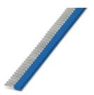
Taped ferrules, 2.5 mm<sup>2</sup>, sleeve length 8 mm, with plastic collar, according to DIN 46228-4, blue, for processing with the CRIMPFOX 4 IN 1, 10 strips each with 40 sleeves per strip.
