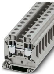
Feed-through terminal block, nom. voltage: 1000 V, nominal current: 76 A, number of connections: 2, connection method: Screw connection, Rated cross section: 16 mm<sup>2</sup>, cross section: 1.5 mm<sup>2</sup> - 25 mm<sup>2</sup>, mounting type: NS 35/7,5, NS 35/15, color: gray
