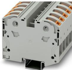
High-current terminal block, nom. voltage: 1000 V, nominal current: 125 A, number of connections: 2, connection method: PowerTurn connection, Rated cross section: 35 mm<sup>2</sup>, cross section: 2.5 mm<sup>2</sup> - 35 mm<sup>2</sup>, mounting type: NS 35/15, color: gray
