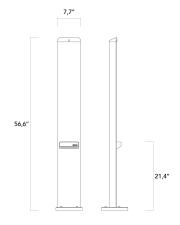
All components of SNOC luminaires are made from aluminum alloy A-356 or A-413 including less than 0.2% copper and resistant to oxidation.
