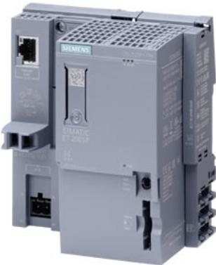
SIMATIC DP, CPU 1512SP F-1 PN for ET 200SP, central processing unit with 600 KB work memory for program and 2 MB for data, 1st interface: PROFINET IRT with 3-port switch, 25 ns bit performance, SIMATIC Memory Card required, BusAdapter required for port 1 and 2
