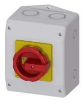
SENTRON, Switch disconnector 3LD, emergency switching-off switch, 3- pole, lu: 63 A, operating power / at AC-23 A 400 V: 22 kW, Molded plastic encapsulation for inch cable gland, rotary operating mechanism, red/yellow
