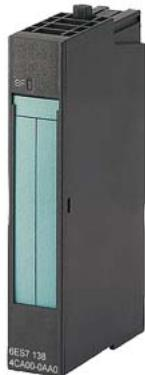
\*\*\* Spare part \*\*\* SIMATIC DP, Electronics module f. ET200S, 2 AO U, 15 mm width, +/-10V; 13 bit+sign, 1..5 V; 12 bit, Cycle time less than 1 ms with SF LED (group fault)
