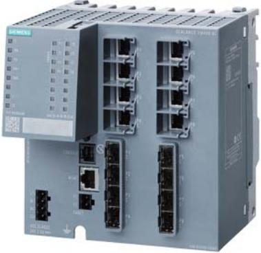
SCALANCE XM408-8C; managed modular IE switch; 8x 10/100/1000 Mbit/s RJ45; 8x 100/1000 Mbit/s SFP; contains 8 combo ports; in total 8 ports can be used; expandable to 24 ports electrical or optical; assembly: DIN rail/S7 mounting rail; PROFINET IO device; redundancy functions; office features (RSTP, VLAN, IGMP,...); C-PLUG in scope of supply; layer 3 with Key-Plug plug available .
