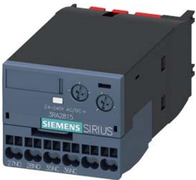
solid-state time-delayed auxiliary switch, off delayed, without control signal, relay 1 NC + 1 NO, time range 0.05-100 s, 24-240 V AC/DC, 50/60 Hz, varistor for attenuation of the contactor coils integrated, spring-loaded terminal, can be snapped onto the front on contactors 3RT20 and contactor relays 3RH2
