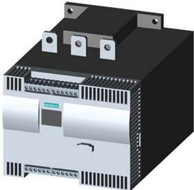
SIRIUS soft starter Values at 575 V, 50 °C standard: 315 A, 300 hp Inside-delta: 546 A, 600 hp 400-600 V AC, 115 V AC Screw terminals !!! Phased-out product !!! Successor is SIRIUS 3RW5, Preferred successor type is >>3RW5546-6HA16<<
