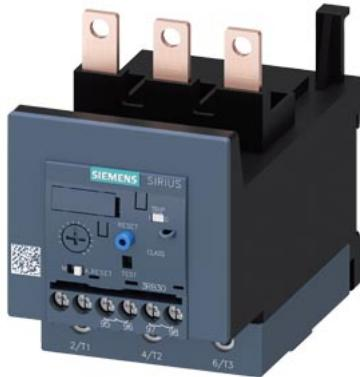
Overload relay 32...115 A Electronic For motor protection Size S3, Class 10E
