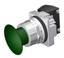
30mm Command/52, Chrome Finish Heavy Duty, Watertight/Oiltight Complete Metal Unit Push-Pull Operator Non-Illuminated Mushroom Head Cap Small 1.73" (44 mm) Metal, Anodized Green 2 Position Maintained, Pull-to-Release with 1 N.O. - 1 N.C. Heavy Duty Contacts, A600/P600 UL Listed, CSA Certified NEMA 1,3,3R,4,4X,12,13 & Automotive Standards
