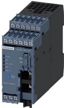
Basic unit SIMOCODE pro V EIP, EtherNet/IP, medium redundancy DLR, Web server, transmission rate 100 Mbps, 2 x bus connection via RJ45, 4I/3O freely parameterizable, Us: 24 V DC, input for thermistor connection Monostable relay outputs, expandable by extension modules
