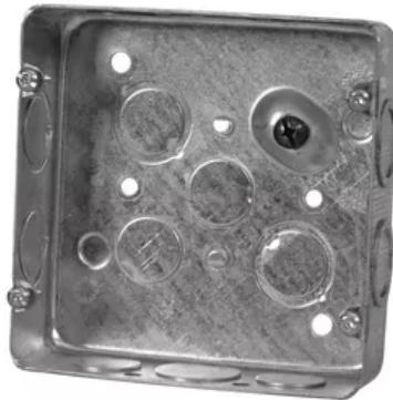
4-11/16 In. Square Box, 1-1/2 in. Deep, 30 Cu. In., with Raised Ground Screw, with Concentric, 1/2 & 3/4 in. KO (30-Pack).
