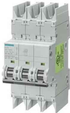
Circuit breaker 10kA, 3-pole, D, 6A according to UL 489-480Y/277V
