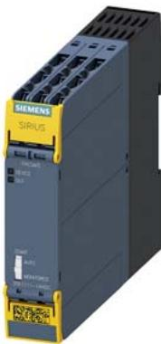
SIRIUS safety relay Basic unit Standard series Relay enabling circuits 3 NO contacts plus Relay signaling circuit 1 NC contact Us = 110 - 240 V AC/DC 50/60 Hz screw terminal
