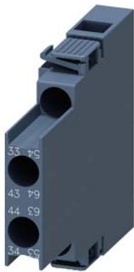
auxiliary switch, lateral, 2 NO, on the left: 33/54, 63/64, on the right: 33/34, 43/44, current path: 1 NO, 1 NO, screw terminal, for contactors 3RT2 and contactor relays 3RH2
