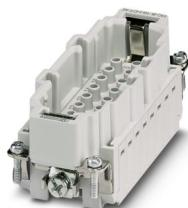
Contact insert, number of positions: 16+PE, size: B16, number of connections per position: 1, Pin, Crimp connection, 500 V, 16 A, 0.5 mm<sup>2</sup> ... 4 mm<sup>2</sup>, application: Power
